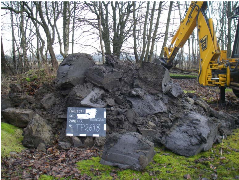
TP2698 – Made Ground (HSTD/MGT2A) over silty clay (LPF).
