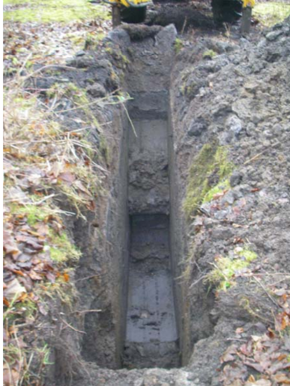
TP2698 – Made Ground (HSTD/MGT2A) over silty clay (LPF).
